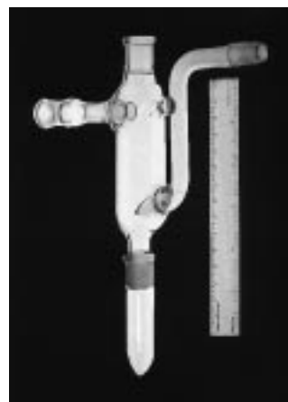
Figure 1. Small-scale apparatus for the distillation of 1a–c from solution in hexadecane. Solutions of 1a–c can be prepared by addition of the desired solvent to the hexadecane solution prior to distillation. The ruler is 15 cm long.
